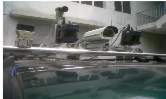
Fig. (2) Sensors mounted on the vehicle
