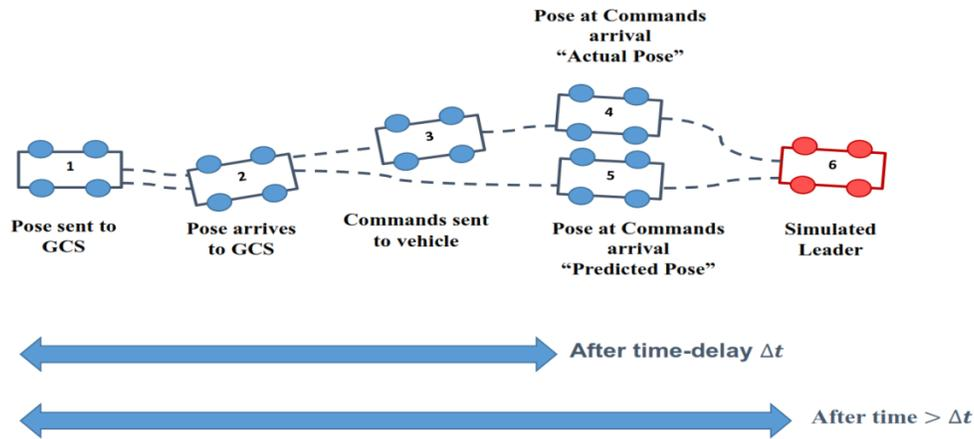
Fig. (3) The predicted vehicle appears in the future after time slightly more than  $\Delta t$ .
