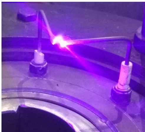
Figure 16: Ignition using LASER igniter in combination with electric spark igniter
