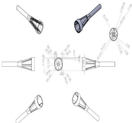
**Figure 5: four slot EV burner.**
