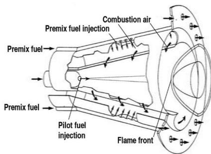
**Figure 4: Two slot EV burner.**
