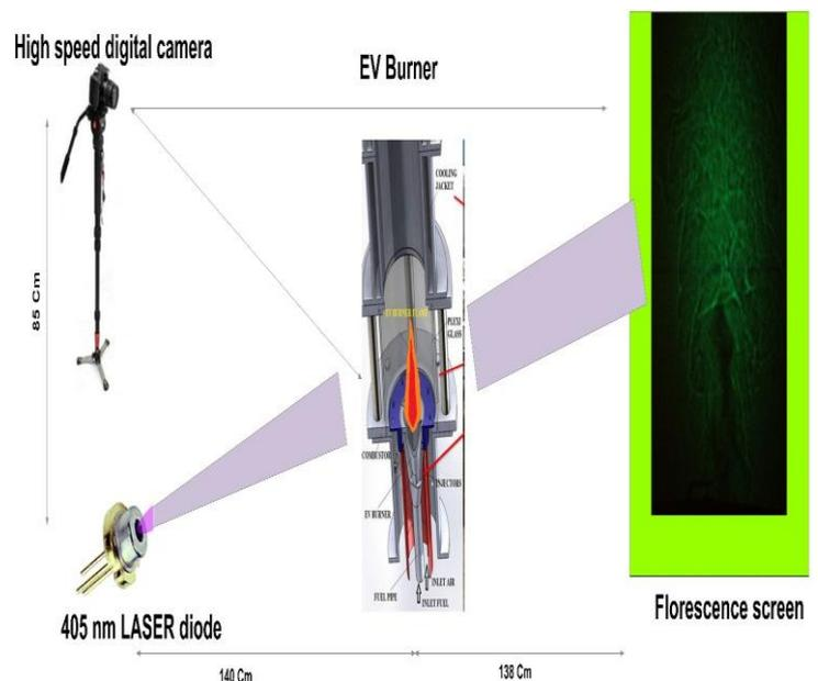
Figure2: Schematic diagram of system set-up
