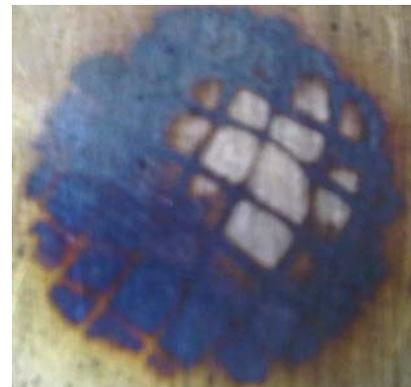
Fig.(11) Photographic picture of copper Faraday cup at optimum parameters for applying positive potential on retarding grid using argon gas.
