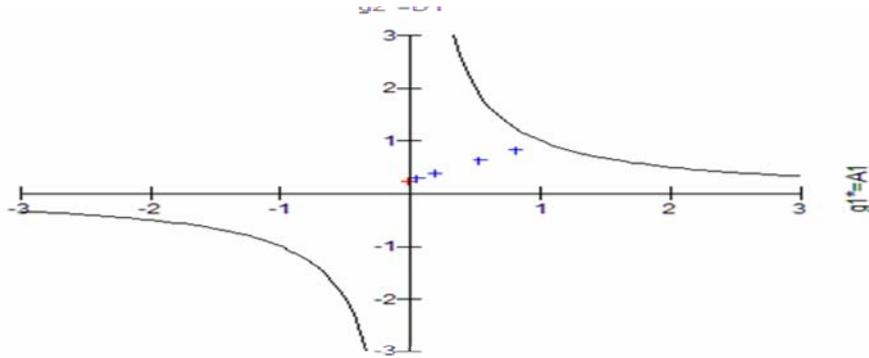
Figure (4) the stability realization of the Nd:YVO<sub>4</sub> designed cavity with (20,40,66 and 75mm) in length (from right to left) and shows the unstable case at the cavity total length above 75mm denoted by the extreme lift cross.
