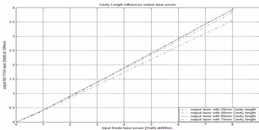
Figure (3) the effect of the cavity length design on the Extract output laser; solid red line was the highest slope efficiency with a maximum extracting laser output up to 3.965 Watt.
