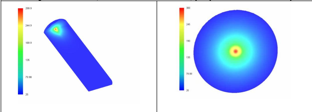
Thermal gradient for 7.8W(focused on the front rod face) pumped 3\*10mm Nd:YVO<sub>4</sub> crystal
