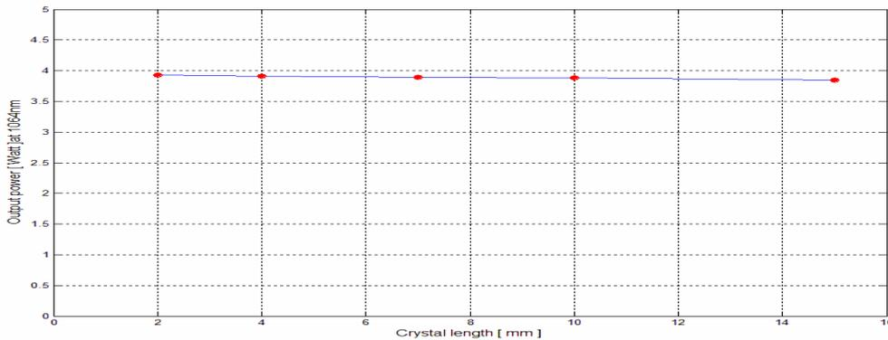
Figure (6) Laser output power Vs. Crystal length curve
