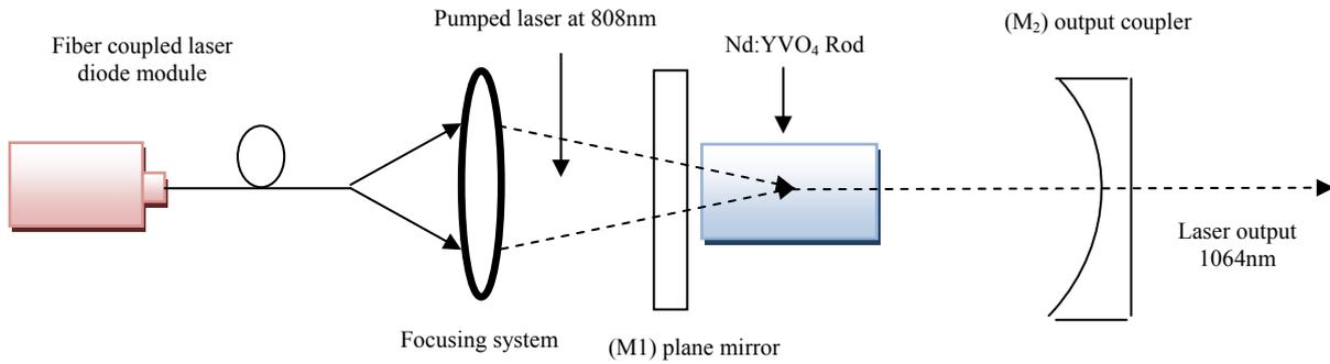
Figure (1) the DPSS Nd:YVO<sub>4</sub> laser with the a single End pumping configuration
